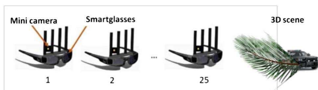
Fig. 4. ADS experimental setup with AR glasses and camera.
