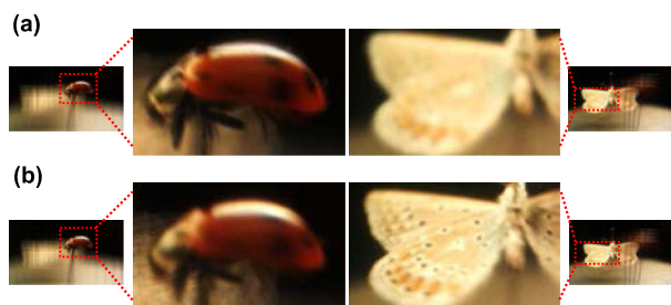
Fig. 4. Experimental results for the 3D SAIL endoscopy with the tunable large-aperture LC lens. The computational reconstruction results of two sets of elemental images under two voltage conditions of the LC lens. (a) (V_1, V_2) = (90 V_{\text{rms}}, 30 V_{\text{rms}}) and (b) (0, 45 V_{\text{rms}}) .
