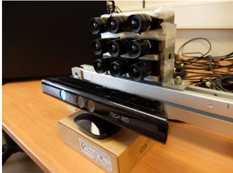
Fig. 2. Two sensors used in the experiments: the 3 \times 3 camera array on top and the Kinect below.
