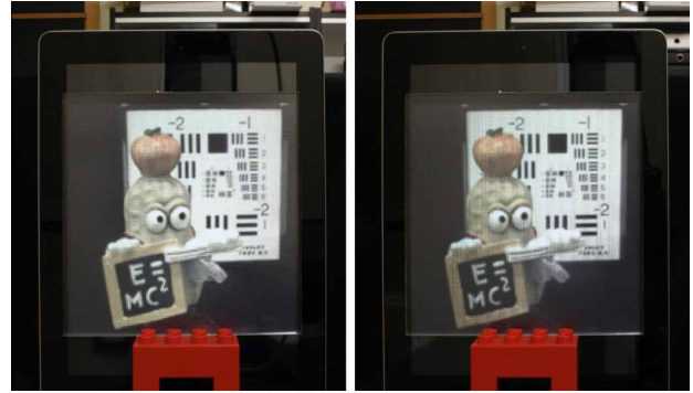
Fig. 14. Two views of the 3-D image as displayed by the IP monitor.
