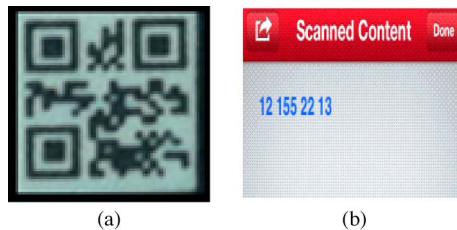
Fig. 2. (a) Enlarged QR code taken using the iPhone 4 camera; (b) scanned QR code depicting the encrypted and compressed data using the iPhone SCAN Application.
