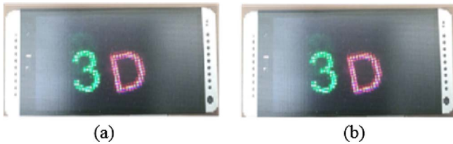
Fig. 6. 3D display results using Smartphone. (a) 3D optical reconstruction with integral imaging using the primary EIs. (b) Optical 3D reconstruction using the decrypted and decompressed EIs obtained from the compressed DRPE EIs in QR codes.
